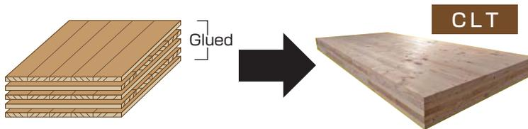
It is used widely primarily in Europe and the United States in the walls and floors of mid-to-high rise buildings and other buildings. It offers freedom of design, and there are various structural types, including the CLT panel construction method mentioned above.
