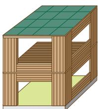
(1) CLT panel construction method
