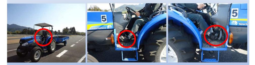
Left: Steering wheel Center: Clutch Right: Brake
