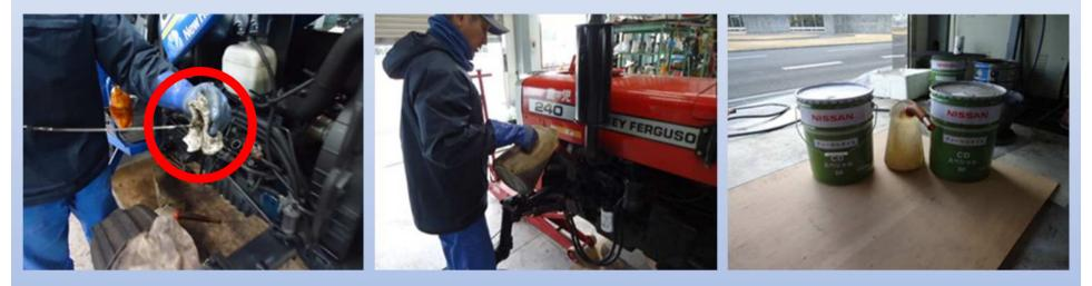
Left: Check the oil level using the oil gauge.
